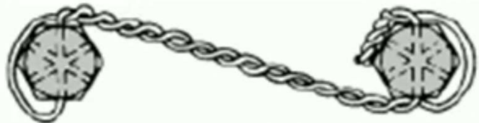
Safety wire Bolt-Heads
